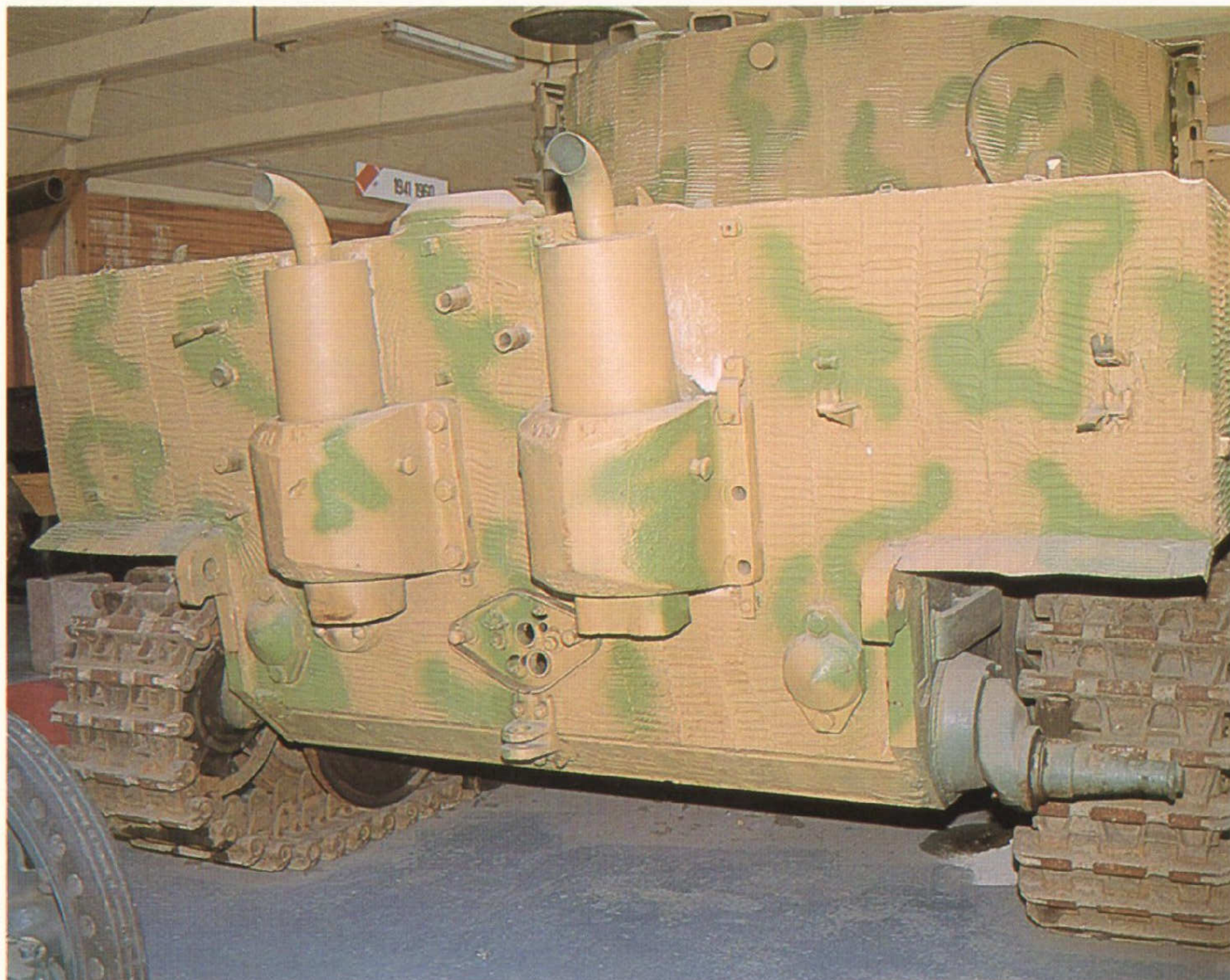
Two heavy cast exhaust manifolds are bolted to the 82mm thick rear plate. Omitted on this museum model are the large metal sheet covers that serve as heat protectors. Located in the bottom corners of the rear hull plate are the track tension access covers.
