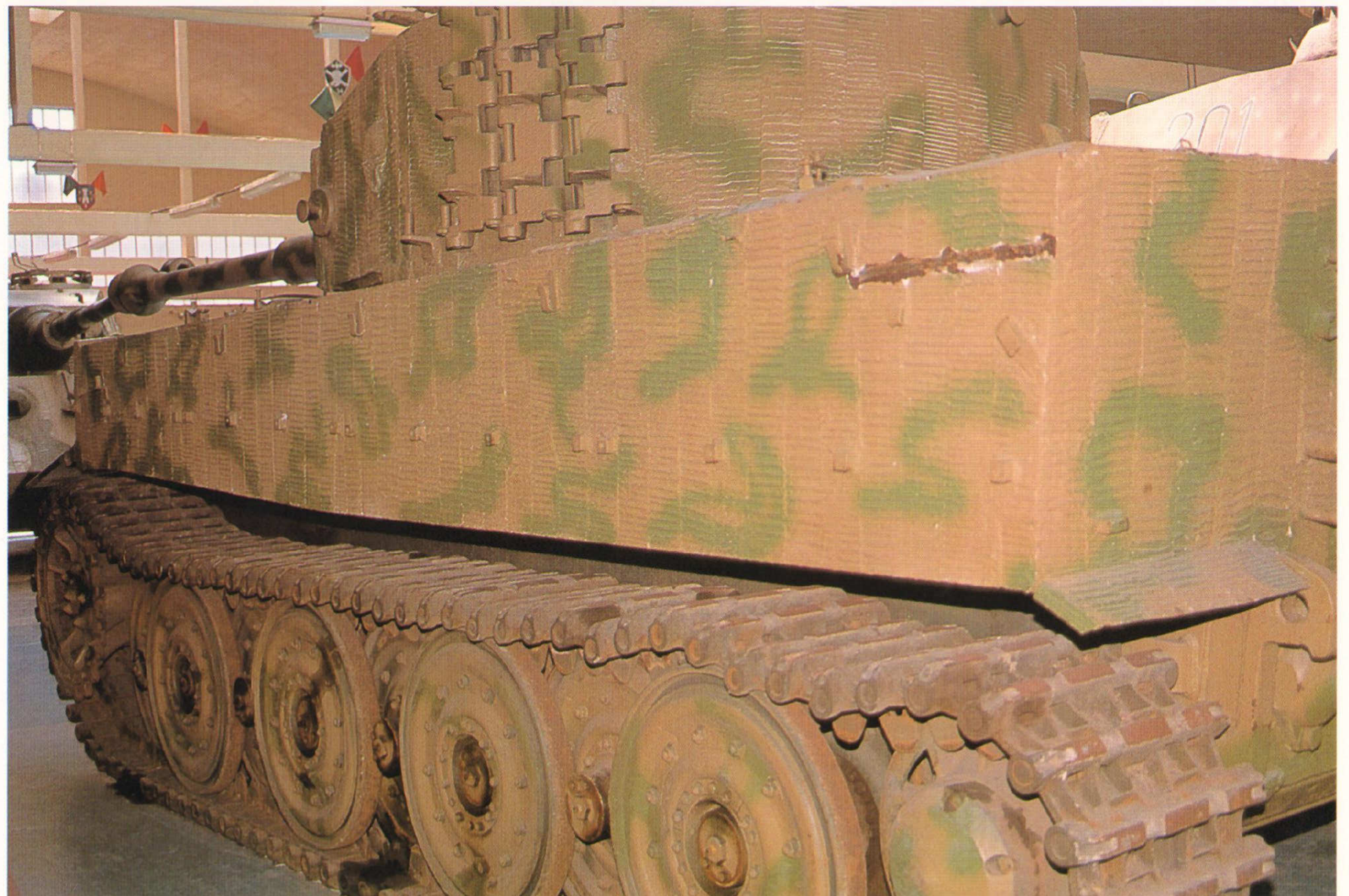
Left hull side showing mounting pads for the side skirts and fasteners for the track cables.
