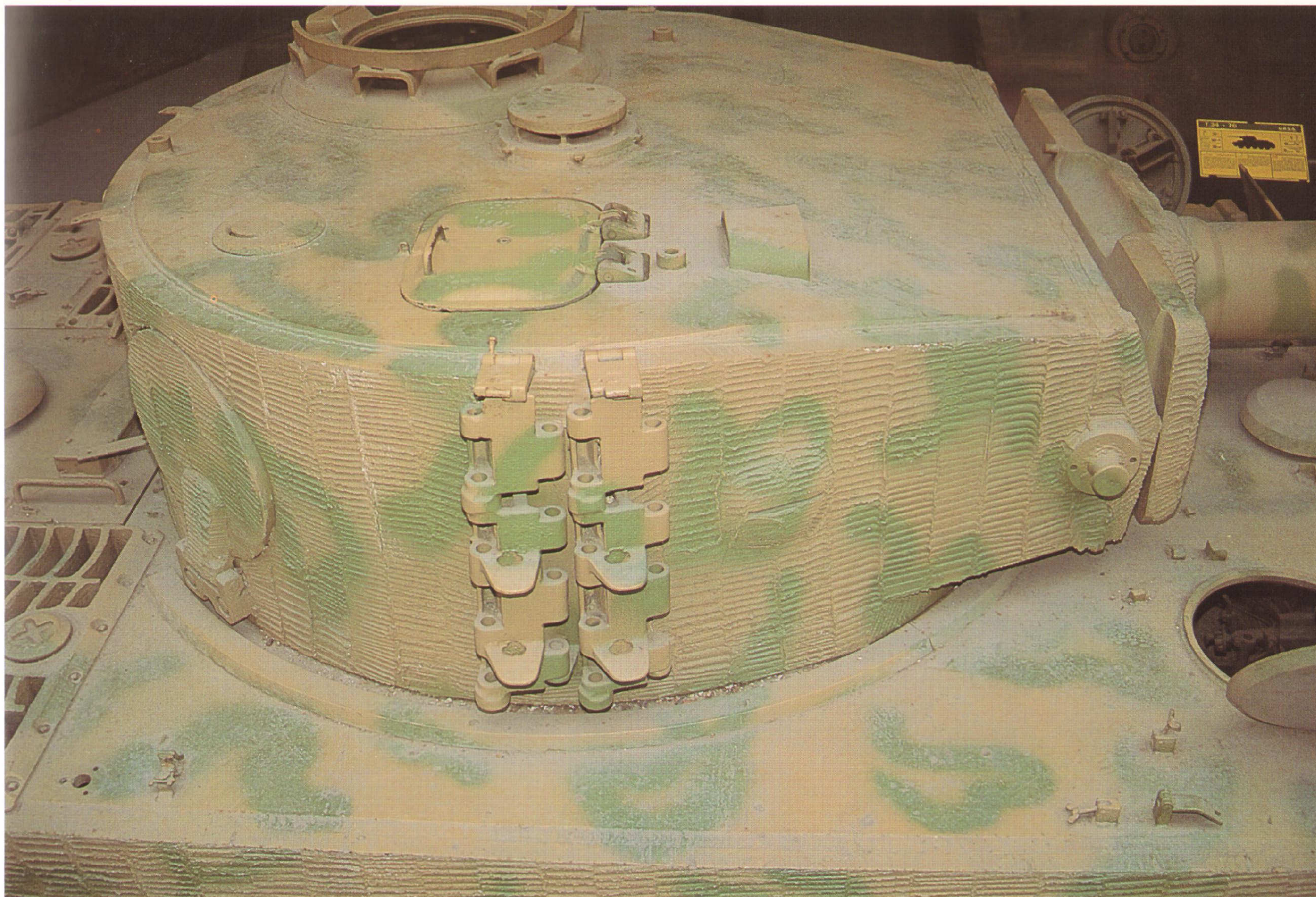
A general view of the turret from the right showing only two spare track links attached to this side. Note the rectangular shape of the loader's hatch closest to the camera and its hinges at the leading edge. The thick armor of the turret side can easily be established from this view. Note the rim surrounding the lower turret edge for side protection of the turret traverse ring. Also apparent is the turret roof ventilator.
