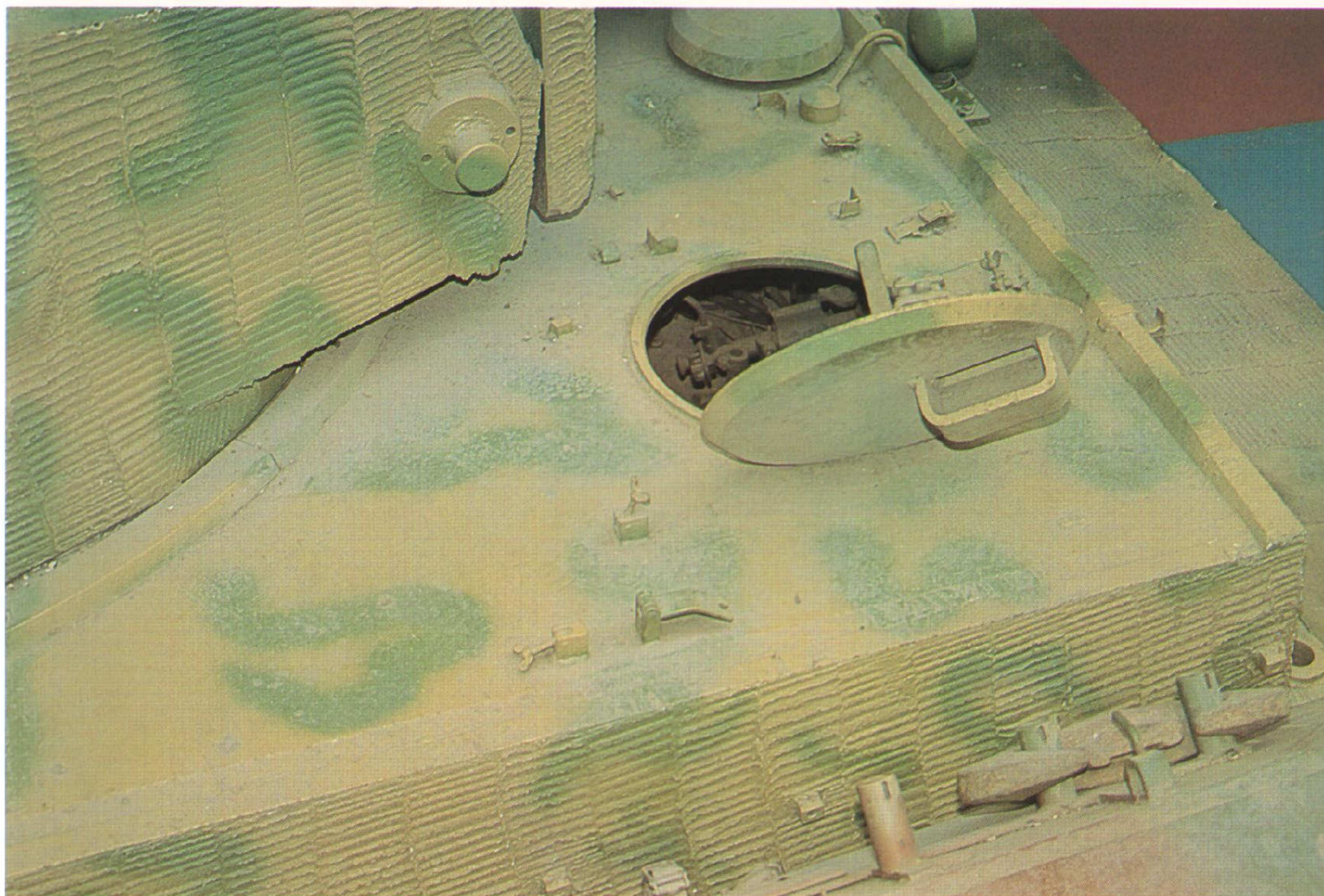
(Above, left & right) View on the radio operator's hatch area at right front of the hull. Note the heavy welding seams of the hull armor plates. The balance spring of the driver's and RO's hatches (enabling easy opening) is welded to the hull roof. Note the episcopes mount and the crank handle opening mechanism.
